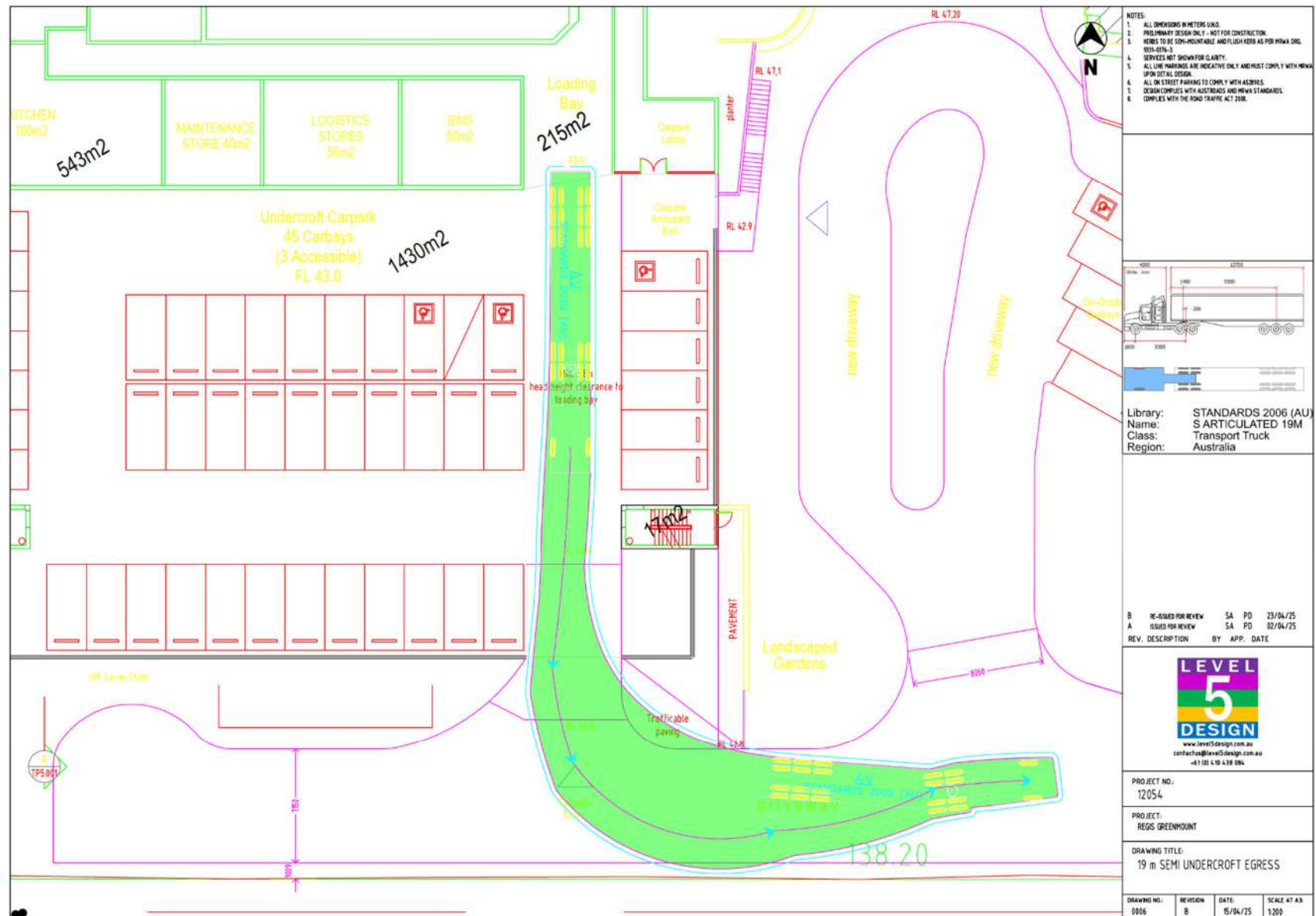
Figure D3 - Swept Path – 19.0 m Articulated Vehicle (AV) Egress
